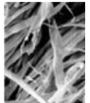
*Fabric squeezed using high-expression rubber roller (1000X magnification)
